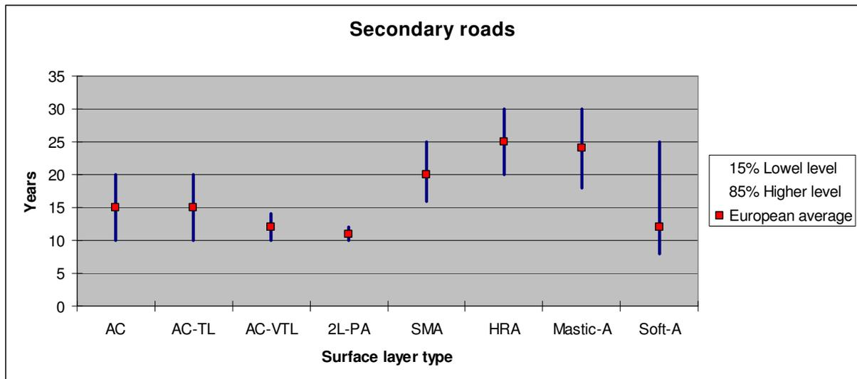
**Figure 9: Durability of surface layers on secondary roads**
