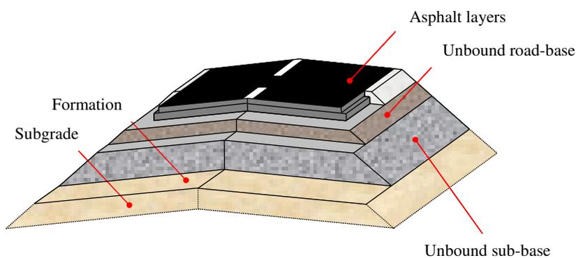
Figure 2. Schematic illustration of flexible pavement structure.
