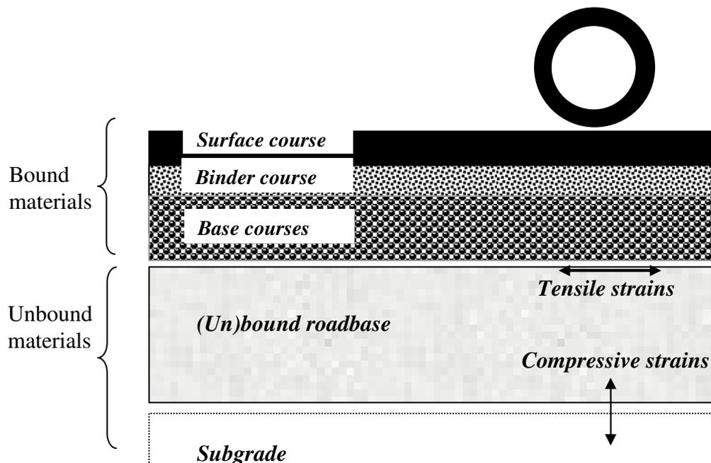
Figure 4. Example of pavement structure and the two traditional design criteria.
