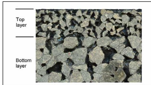
Figure 5: Structure of Double layered Porous Asphalt
