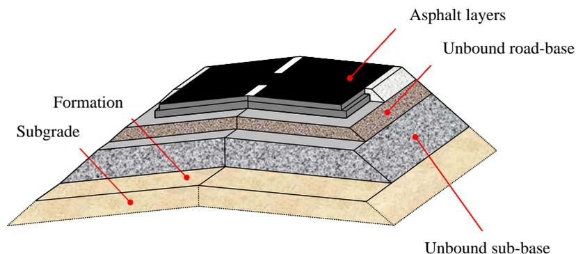
Figure 1. Schematic illustration of flexible pavement structure.
