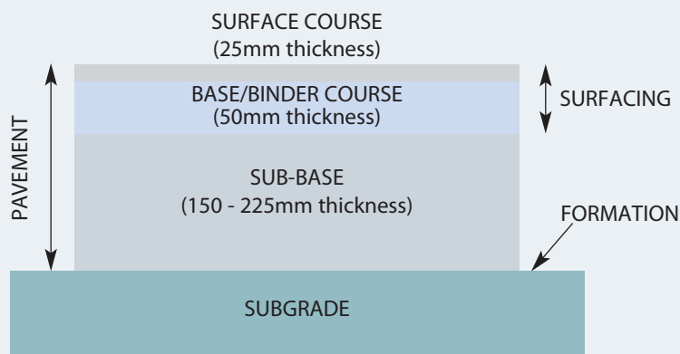
Figure 2b 'Light vehicle category pavement thicknesses'
