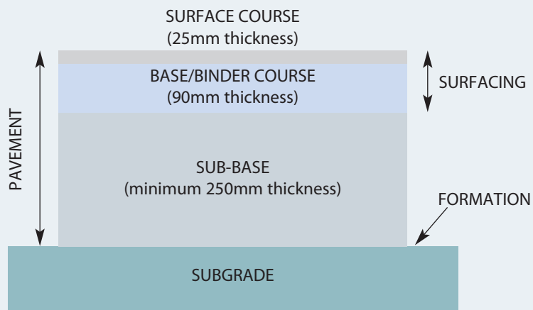
Figure 2c 'Heavy vehicle category pavement thicknesses'
