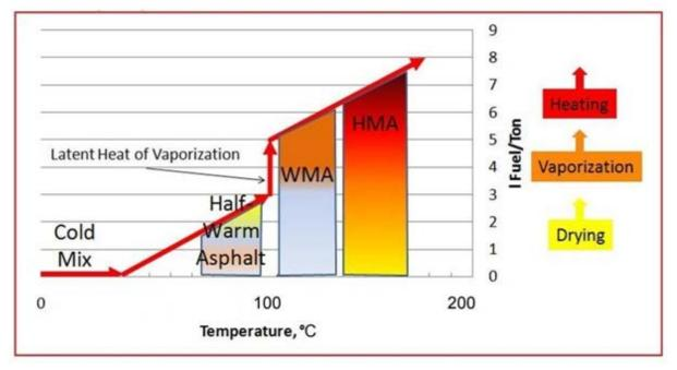
*Figure 1: Classification by temperature range (Temperatures, and fuel usage are approximations) [1.]*
