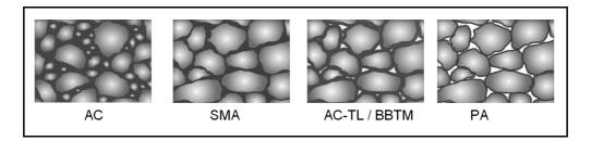
Figure 5: Difference in structure between AC, SMA, BBTM and PA.
