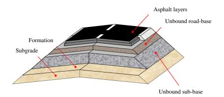
Figure 2. Schematic illustration of flexible pavement structure.
