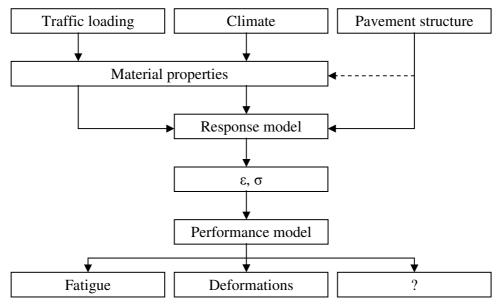
Figure 3. Schematic illustration of semi-mechanistic design method.
