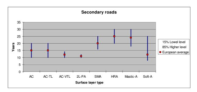
Figure 9: Durability of surface layers on secondary roads
