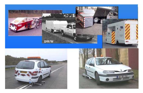
Figure 2.5: Trailer or car-based CPX equipments
