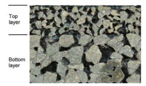
Double layered porous asphalt
