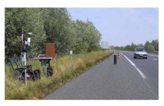
Figure 2.4: Statistical Pass-By measurements
