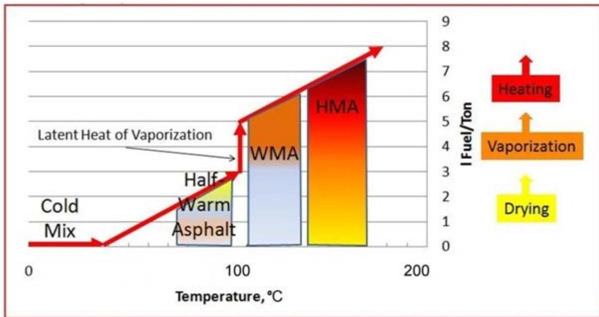
*Figure 1: Classification by temperature range (Temperatures, and fuel usage are approximations) [1.]*
