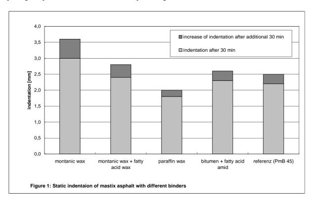
The reference mastic asphalt was produced with a temperature of 250°C. Only a combination with paraffin wax provides a substantial improvement in the resistance against permanent deformation vis-à-vis the reference mastic asphalt. A slight or substantial deterioration can be noted in all of the other cases.
