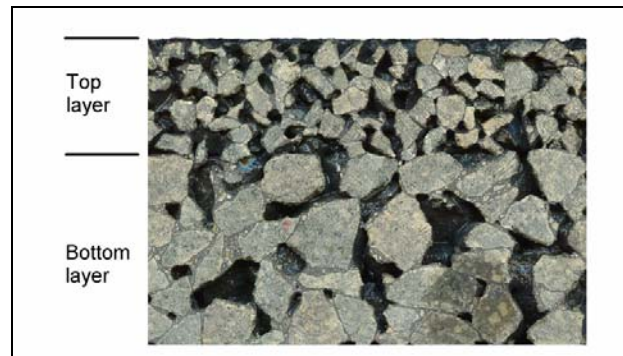
Figure 5: Structure of Double layered Porous Asphalt
