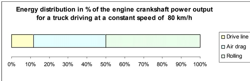
**Figure 9 - Energy distribution of the actual power output of a heavy truck driving at a constant speed of 80 km/h on an even road. [5] Linköping University**
