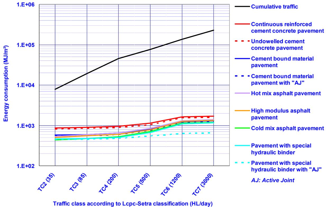
**Figure 5bis - Energy consumption for different types of pavement structure (construction + maintenance of the pavement and safety barriers), compared with the consumption of total cumulative traffic [16]**
