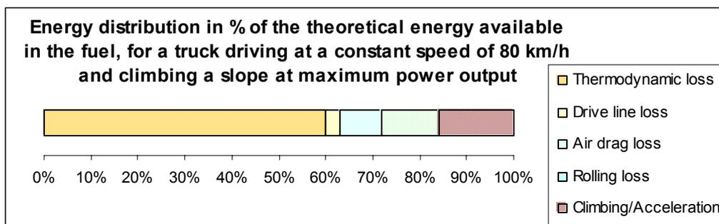
**Figure 8 - Energy distribution of the potential energy available in the fuel**
