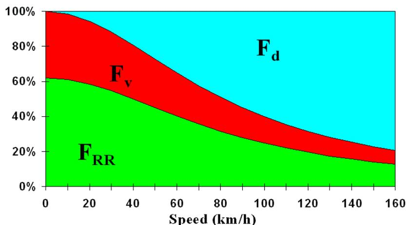
**Figure 10 - Energy distribution in a passenger car versus speed as a percentage of the available power output at the crankshaft**
