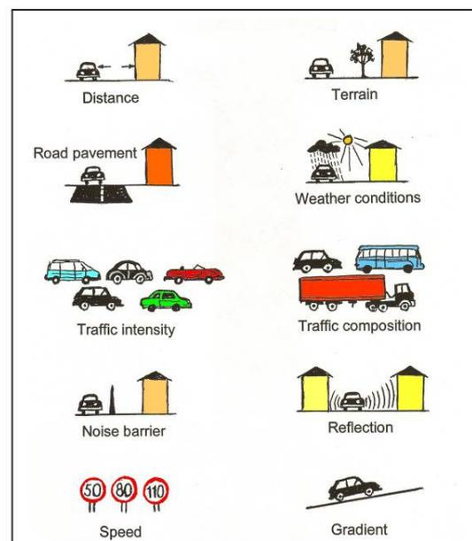
Figure 2.2. Parameters affecting road noise.
