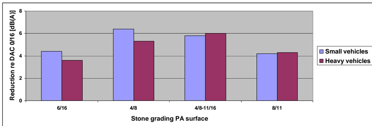
Figure 3.2. Noise reductions of 4 types of porous asphalt concrete relative to dense asphalt concrete (DAC) 0/16 mm.
