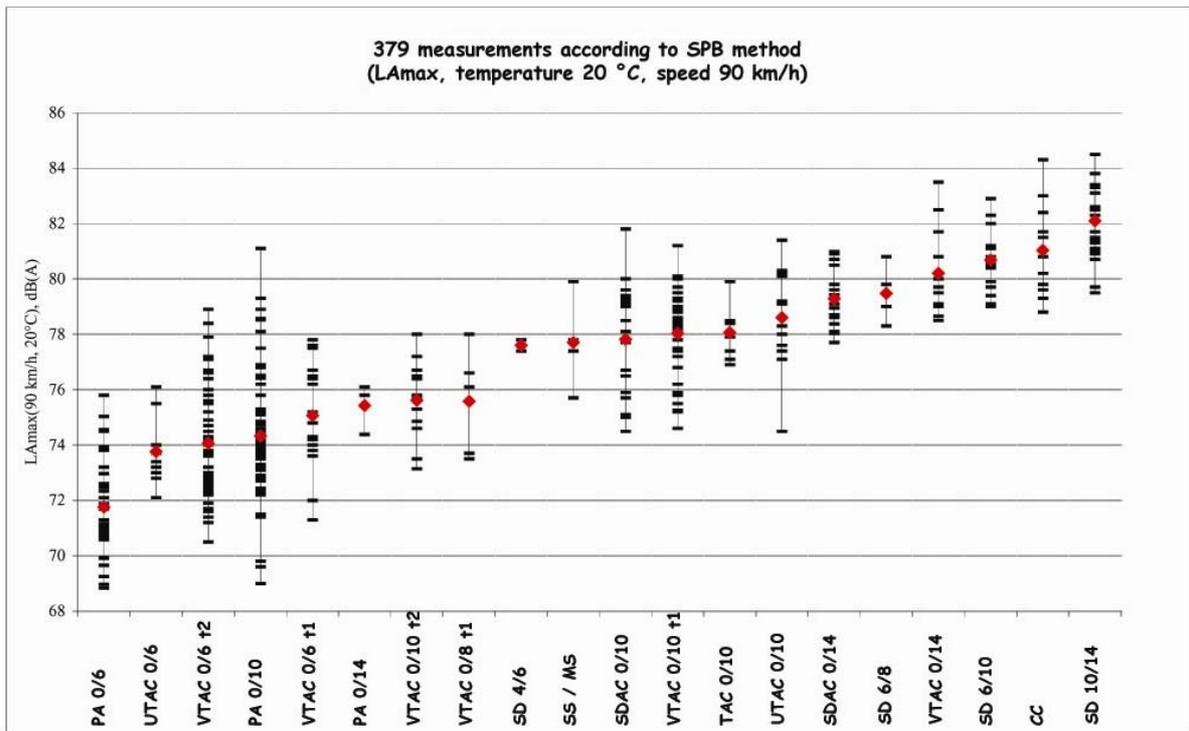
Figure 3.1. Noise levels for different types of overlays [19].
