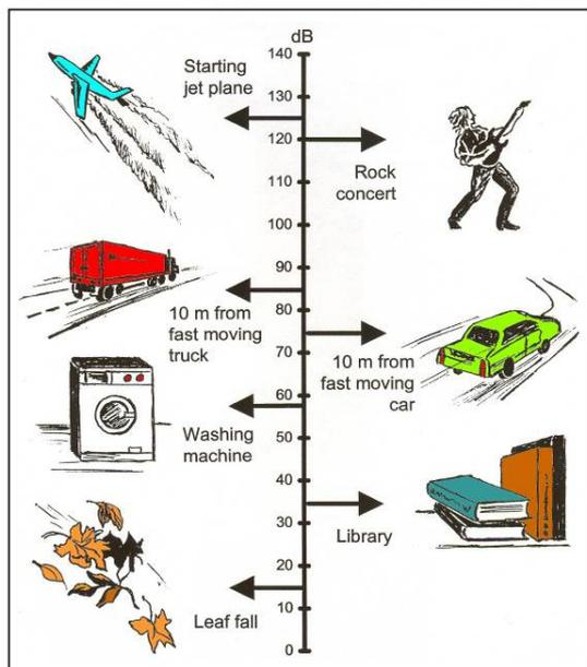
Figure 2.1. Typical noise levels from different traffic sources.
