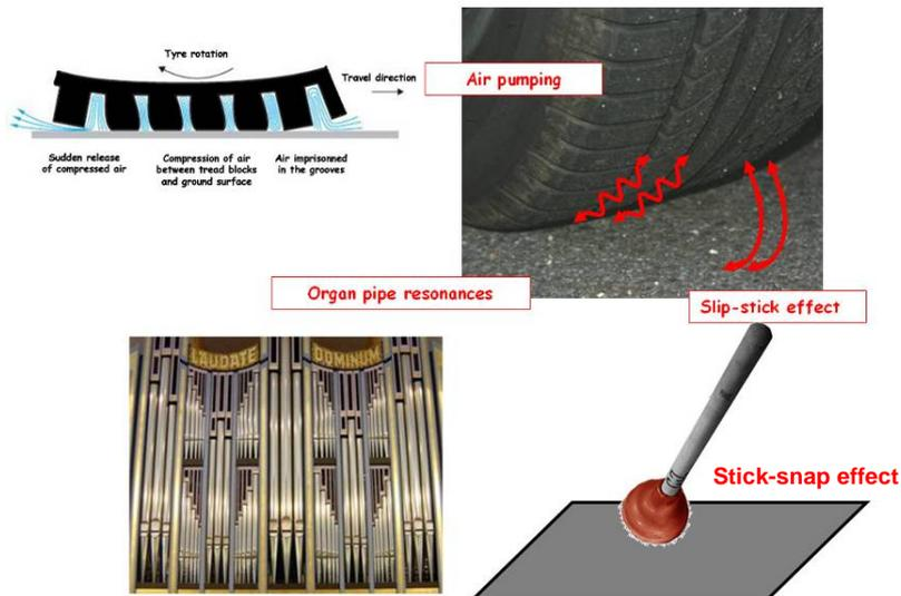
Figure 2.7. Tyre road noise generation mechanisms
