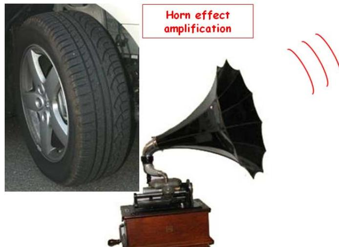
Figure 2.8. Amplification by “horn-effect”
