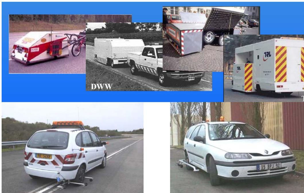
Figure 2.5: Trailer or car-based CPX equipments
