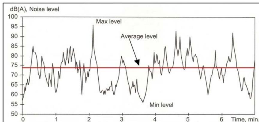
Figure 2.3. Noise level as a function of time and time-averaged measurements
