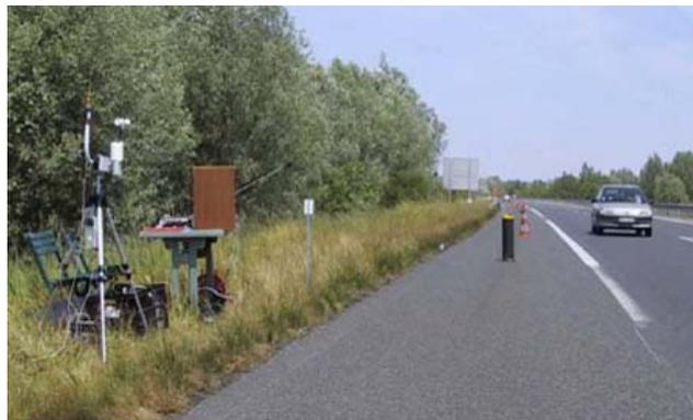
*Figure 2.4: Statistical Pass-By measurements*
